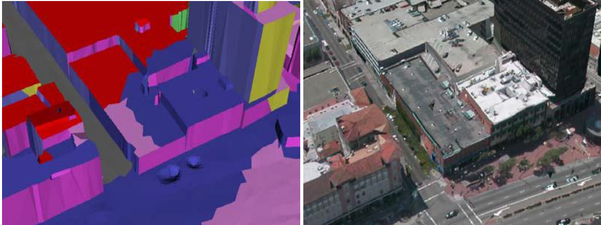
Figure 5. Close-up view of an area texture-mapped with multiple images (a) Source images color-coded; (b) textures applied to the model.
