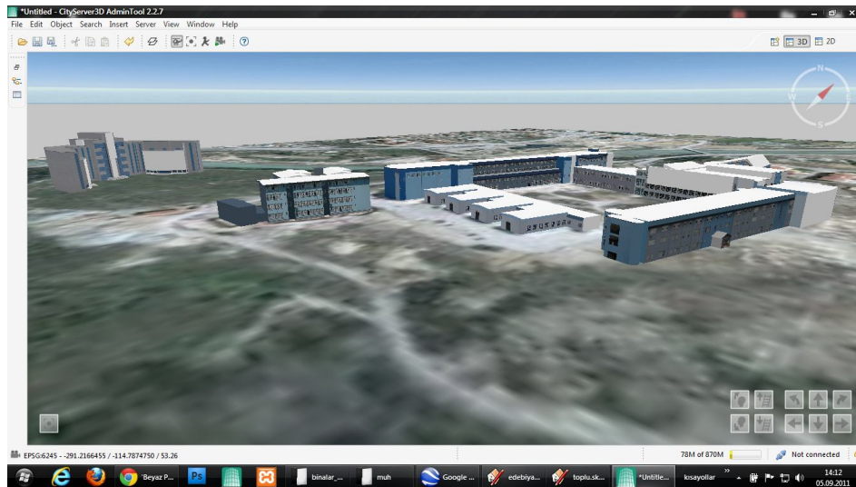
Figure 7: WebViewer of CityServer3D showing a 3D city model with LOD 1
