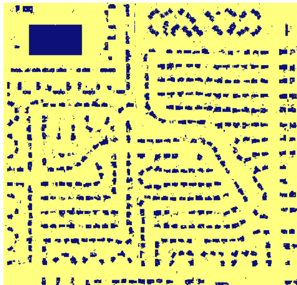
Fig. 3. Output of the neural network model based on chunk processing. The map illustrating the extracted building footprint from the high resolution satellite images
