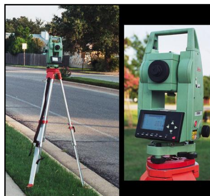
Figure 2. Modern theodolite (Total station)
