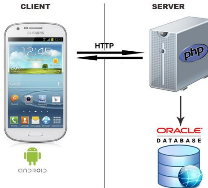
Fig. 2 Architecture of the navigation system
